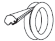
COIL DIRECTION OF REVERSED Q-LON 9941 PT No. 02799310/2 (WHITE / BLACK)
